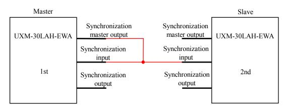
Synchronization output of the master sensor is connected to the synchronization input of the master itself and to the synchronization input of all slave sensors.
